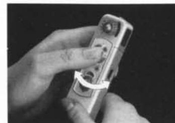
Place thumb on shutter speed dial, hold index finger under camera, turn camera with other hand.
